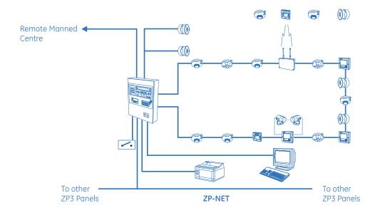
Wired analogue sensors/devices Radio analogue sensors/devices Thermal sensors Smoke sensors Combination sensors High-sensitivity aspirating sensors Volumetric beam sensors Loop sounders Loop relay Loop interface units Loop isolators Callpoints Local and remote I/O Data ports Remote display units and mimics Colour graphic computers and printers
