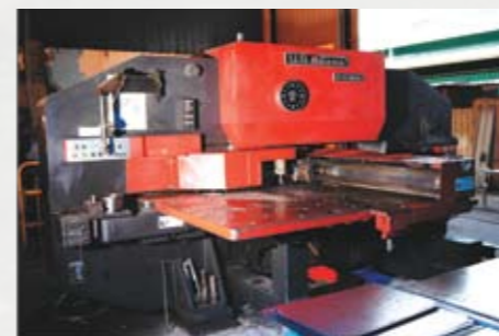
Fabricating of steel cabinet with CNC press brake and CNC turret punch
